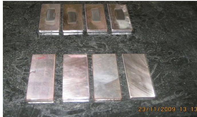
Figure 1. Standard test specimen of size 75mmX 26mmX6mm
